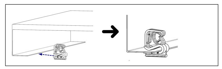
1.2 Insert the latch from the **back side** and secure the main clip to the panel
