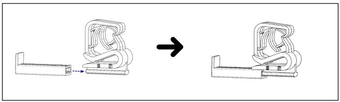
2.2 Press the pre-assembly toward the panel edge, and tighten the latch.
