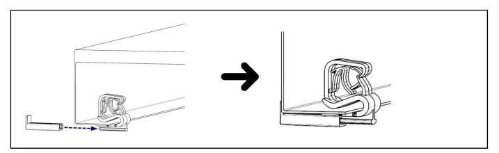
1.3 Press the cable in and it will be clamped.
